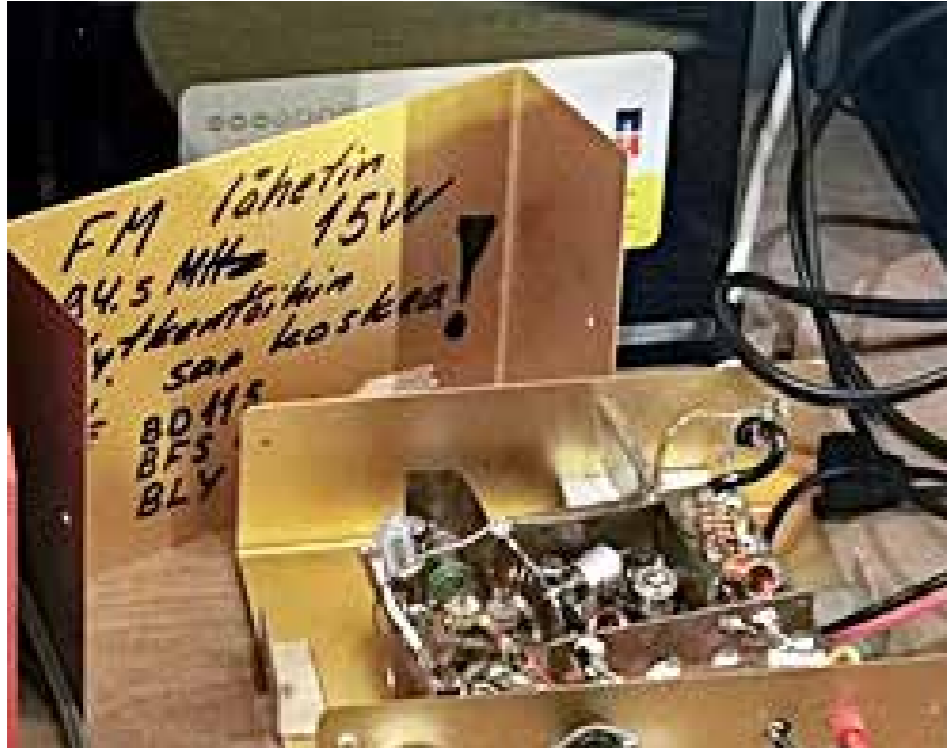
A 15 W FM-transmitter used in pirate radio in Tampere in the 80ies
